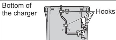
Fasten the AC adaptor cord to prevent it from being disconnected.
